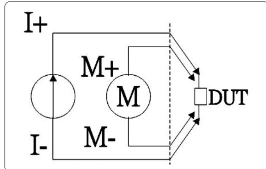
4-wire measurement, avoiding the resistance issues caused from adapting the fixture wires, low resistance of  $1\text{m}\Omega$ .
