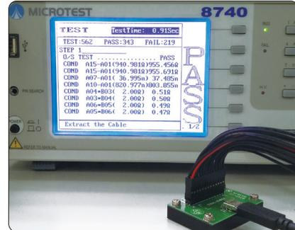
NAC model has four connector loops status; the cable tester will automatically determine the loop status.
