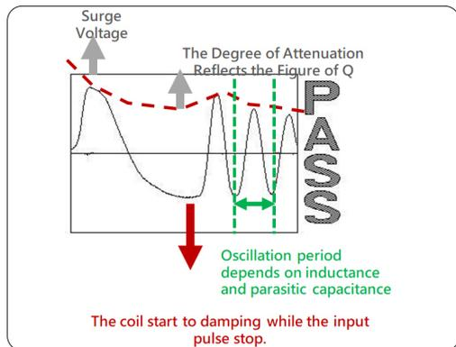
Detect Layer Short by Compare Damped Oscillation Waveforms
