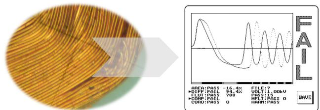
Impulse winding tester inspect by waveform comparison technology. Inspect quality by Damping Attenuation Waveform. The tester offer 200V-3000V impulse voltage to test the DUT. Compare the golden sample waveform.
